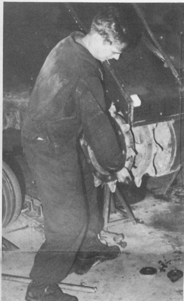
MAKING IT WORK—PFC Robert Bowling, 2nd Battalion, tracked vehicle mechanic changes a drive sprocket on an armored personnel carrier. (Photo by Willie Allen)
