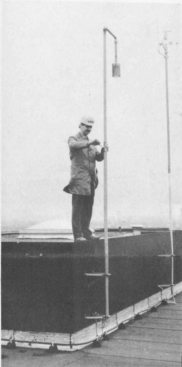
ALL EARS —This small device is called a precision impulse sound level meter EZGA 2. This device picks up aircraft noise and transfers it through telephone cables to the computer center at Tempelhof Central Airport.
