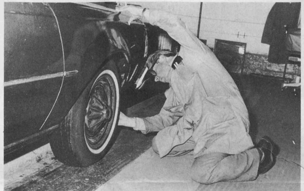
LOOKING FOR TREAD WEAR— The amount of tread on the tires of an automobile can be the determining factor in an emergency situation. And
