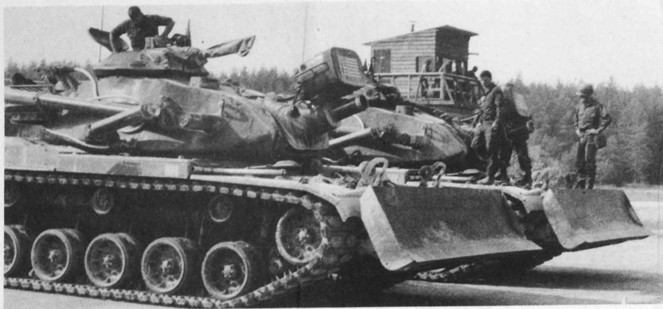
STANDING TALL—42nd Engineers show off their big guns. The Combat Engineer Vehicle comes equipped with a dozer blade and boom as well. The
