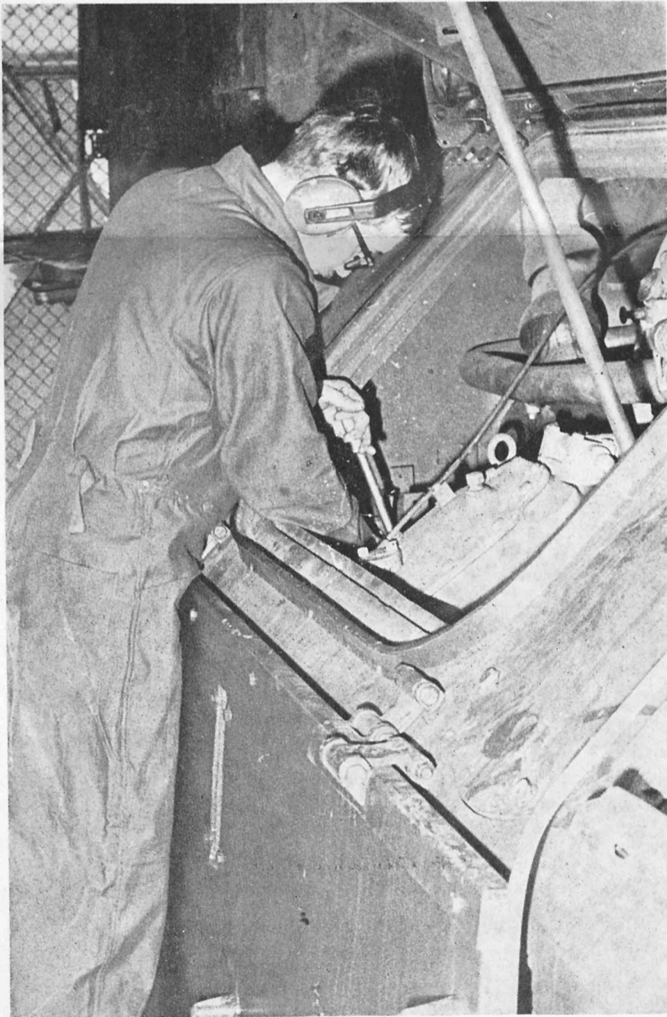
FIXIN' IT — Sgt. Steven Zimmermann, Headquarters and Headquarters Company, 2nd Battalion replaces a universal joint on an M-125A1.
