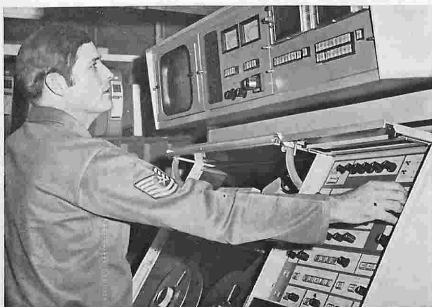
MONITORING THE ABR-1 VIDEO TAPE MACHINE is TSgt. Clyde Brazell, chief maintenance supervisor and member of the 1946 Communication Squadron. This fully computerized machine trouble shoots itself and allows instant analysis of studio productions before they are aired for viewing.
