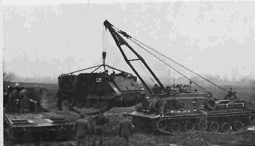
THE VTR LIFTS THE APC TOWARD THE FLATBED.
