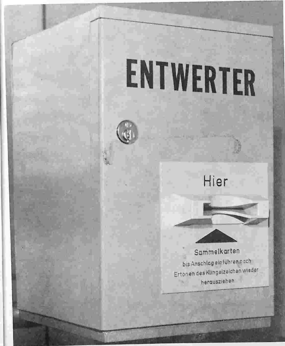
AN ENTWERTER is a red machine which will automatically cancel an Umsteiger or a Sammelkarte. Entwerters are frequently found in U-Bahn stations and are becoming increasingly common on buses. Buses equipped with Entwerters have a bright red sign placed in the right windshield. The instructions tell you to push the ticket into the machine until the bell sounds, and to then withdraw the ticket. (Photo courtesy of BVG)
