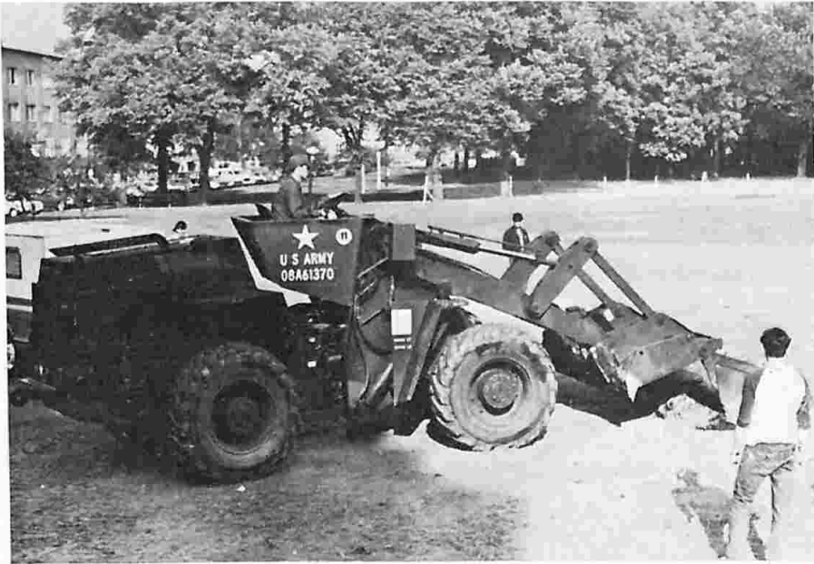
THE FRONT END loader, driven by SP4 "Foggy" Zimmerman of 42nd Engineers, dumps dry dirt on the infield at Andrews. (Photo by Vincent A. Drosdik, III)
