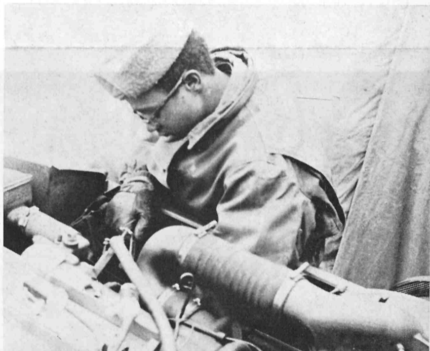
DEFENDER MAINTENANCE PLATOON member, Specialist Four Jerry King repairs the engine of a 2½-ton truck.
